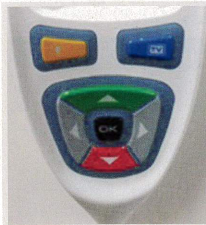
Figure 1. This bedside controller is a clamshell design, the lower half being a two-shot part. The primary shot on the lower part of the body is PC/ABS, and the second shot a seal in TPE. The upper portion of the controller (the part that is invisible in the picture) is a single-shot part also in PC/ABS. The keys are made using the in-mold design (IMD) process. The keys are printed, thermoformed, trimmed, and back injected with PC/ABS. The film is PC. The final step in the process is insert molding the single-shot top. The keys are then inserted into the mold, and a TPE seal is molded around them (this is the gray material between the keys and the white top). The TPE is flexible enough to allow the keys to be depressed to activate the audiovisual system in the room. This is a good example of creative use of IMD being integrated into an active portion of the product. The key tops are durable and bright, and the graphics are behind a protective layer of polycarbonate. The final operation of insert molding the keys to the body is an elegant way of providing good key travel and a water-resistance interface. Courtesy of Yomura
